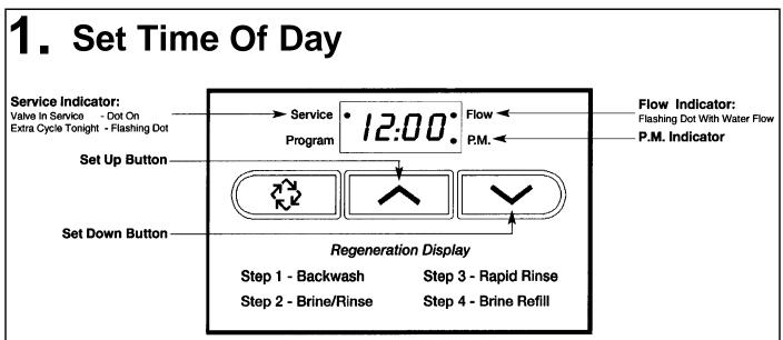
Push either the Up or Down Set Button once to adjust Time Of Day Display by one digit. Push and hold either Up or Down Set Button to adjust Time Of Day Display by several digits.
