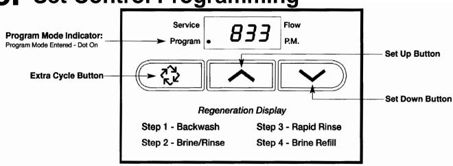
The first option setting display that appears in the Program Mode is Treated Water Capacity. Using the Set Up or Down Buttons, set the amount of treated water that can flow through the unit before a regeneration is required. For Example:
