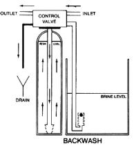
The backwash cycle position directs water to flow down through the riser tube and up through the resin bed and to drain. Foreign material and resin fines are flushed from the mineral tank during this cycle to prepare the resin bed for brining.
