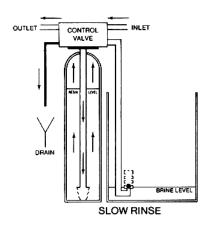
The slow rinse cycle position directs a slow flow of water down through the riser tube and up through the resin bed to drain. This slow flow of water pushes the brine solution through the resin bed
