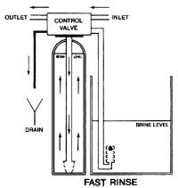
The fast rinse cycle position directs water to flow down through the riser tube and up through the media bed and to drain. Foreign material is flushed from the mineral tank during this cycle.
